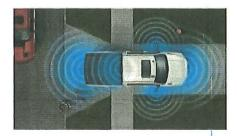
An external backup alarm sounds when the vehicle is shifted into reverse.
